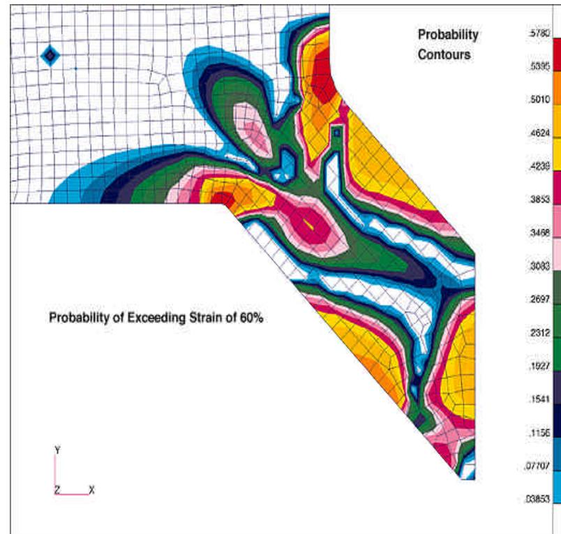
(\*). **Characterization of the Deformed State at Detonation is the “Initial & Boundary Condition” for the Physics Designers.**
