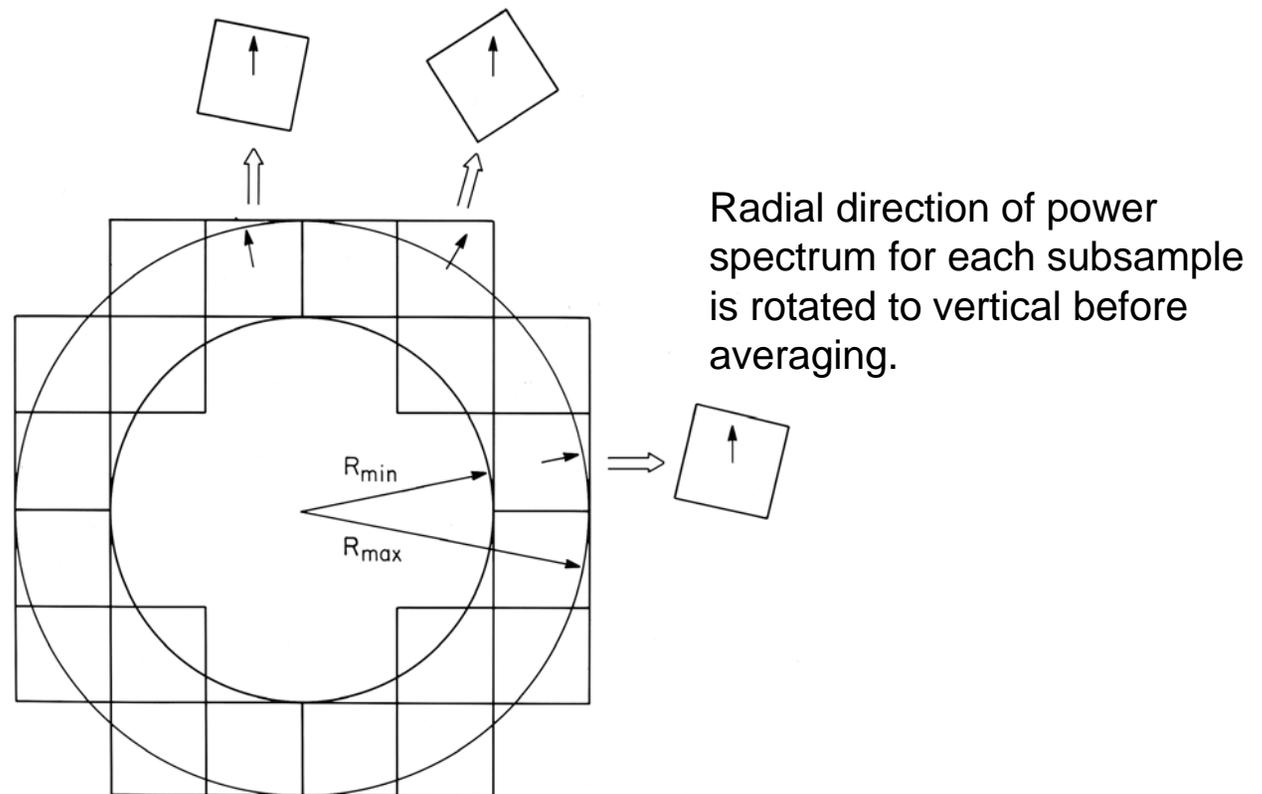
Method of estimating of radial and tangential components of NPS:
