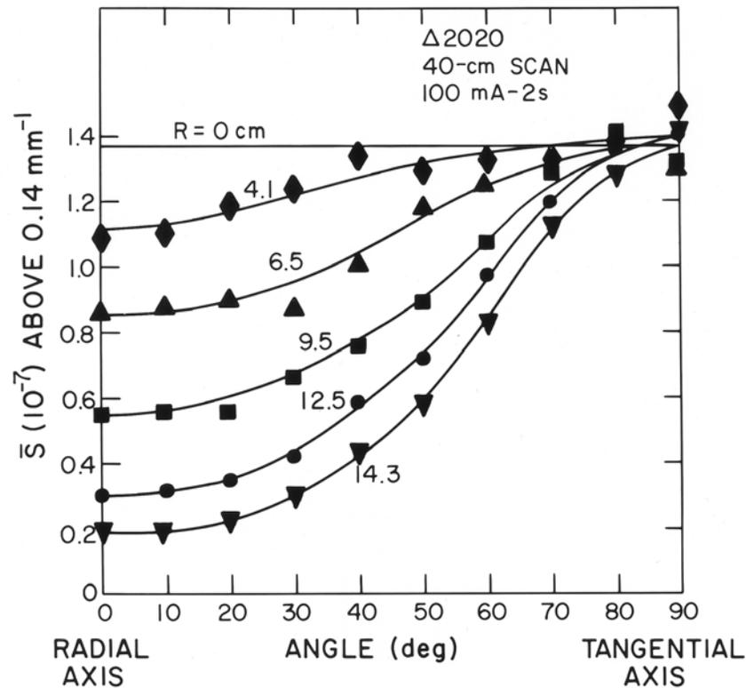
NPS analysis of a Delta 2020 scan of a 35.5-cm-dia water phantom
