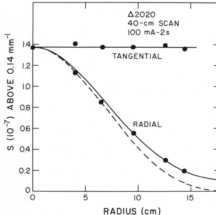
NPS analysis of a Delta 2020 scan of a 35.5-cm-dia water phantom
