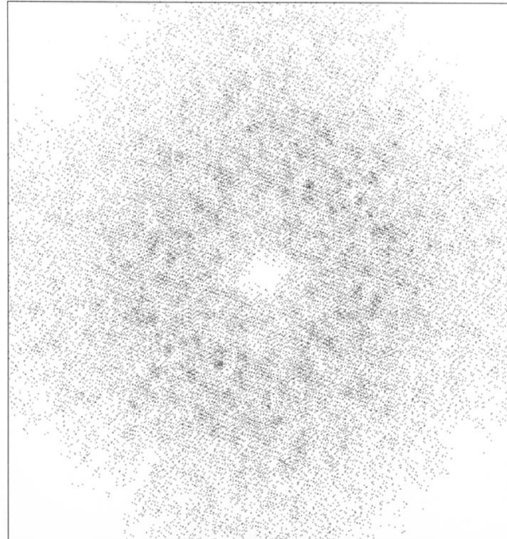
2D NPS for Delta 2020 displayed as a pseudo-grayscale image vs. horizontal and vertical spatial frequency. Zero frequency is in middle of image.
