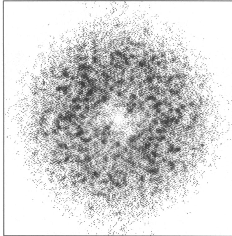
2D NPS for GE 8800 in **full-scan mode** (576 views), displayed as a pseudo-grayscale image vs. horizontal and vertical spatial frequency. Zero frequency is in middle of image.
