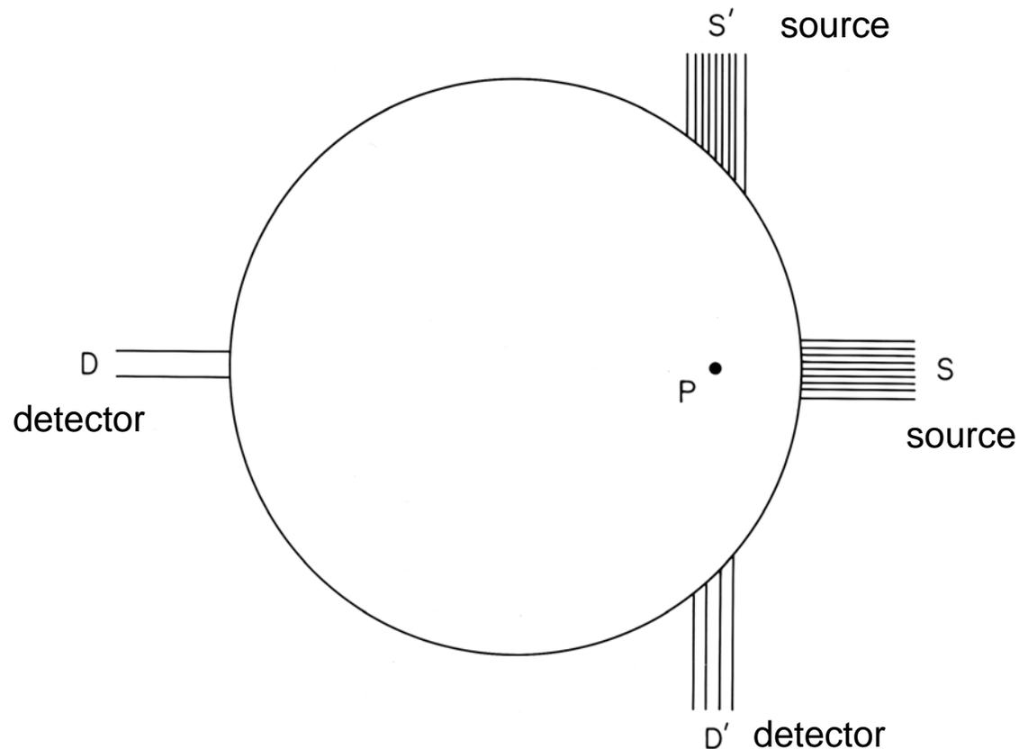
For the same incident x-ray fluence, the transmitted fluence is larger in the tangential direction (S' - D') than in the radial direction (S - D). Thus, one expects the noise at point P in the CT reconstruction to be anisotropic.
