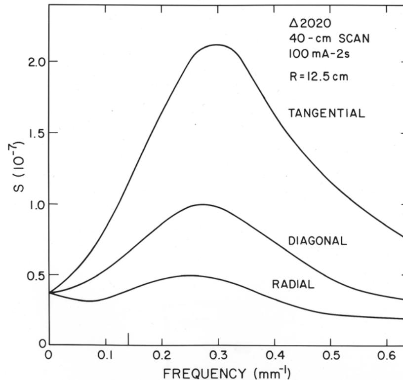
NPS analysis of a Delta 2020 scan of a 35.5-cm-dia water phantom
