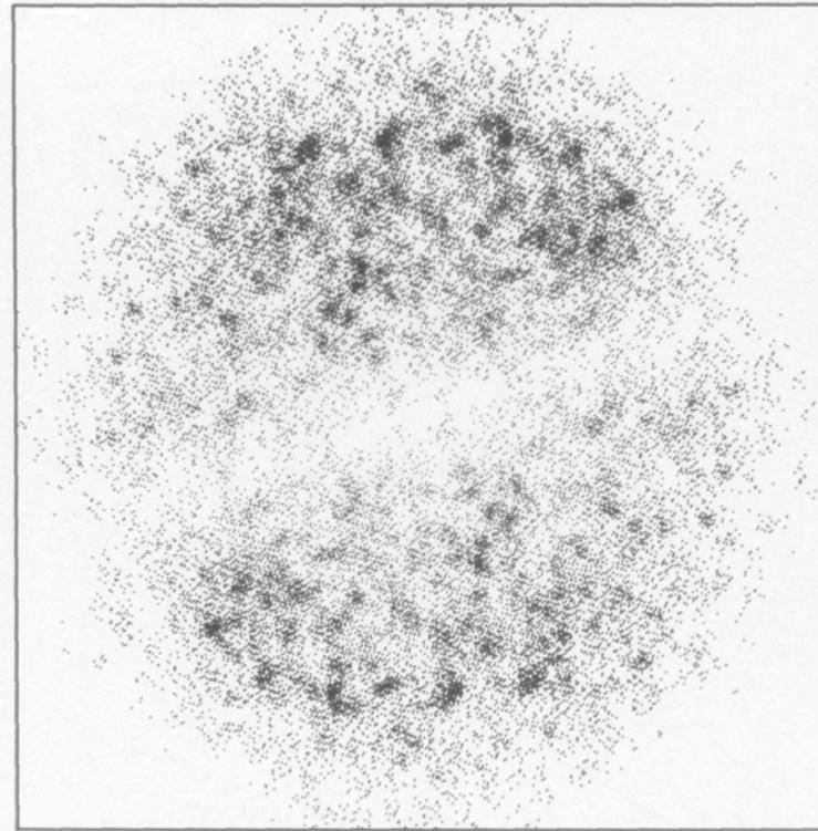
2D NPS for GE 8800 in **half-scan mode** (342 views), displayed as a pseudo-grayscale image vs. horizontal and vertical spatial frequency. Zero frequency is in middle of image.
