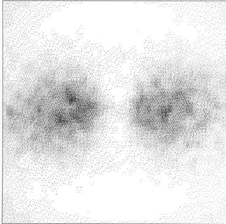
Delta 2020 NPS displayed as a pseudo-grayscale image displayed in terms of the radial (vertical axis) and tangential frequency (horizontal axis). Zero frequency is in middle of plot.
