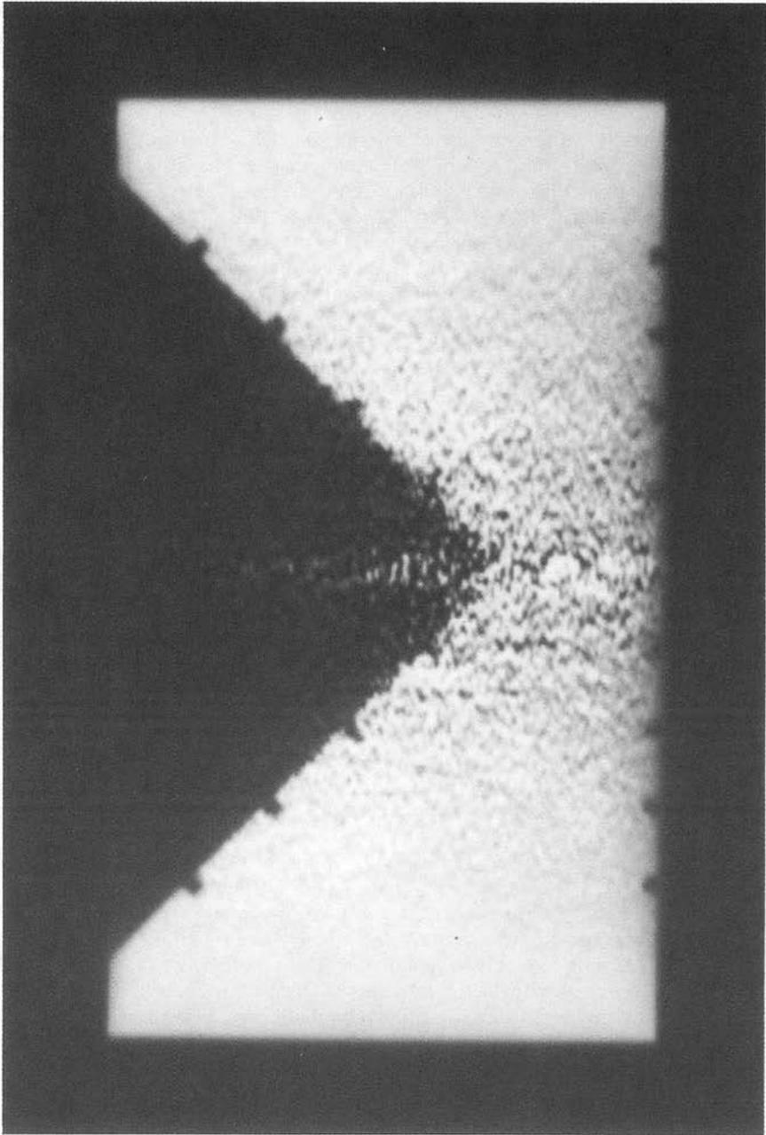
**Fig. 3b** Reconstruction of the cross section of the object derived from Fig. 3a. The  $2 \times 2$ -mm grooves machined in the inner cone and on the end face are much more readily visible. These grooves were nearly invisible in the original radiograph.
