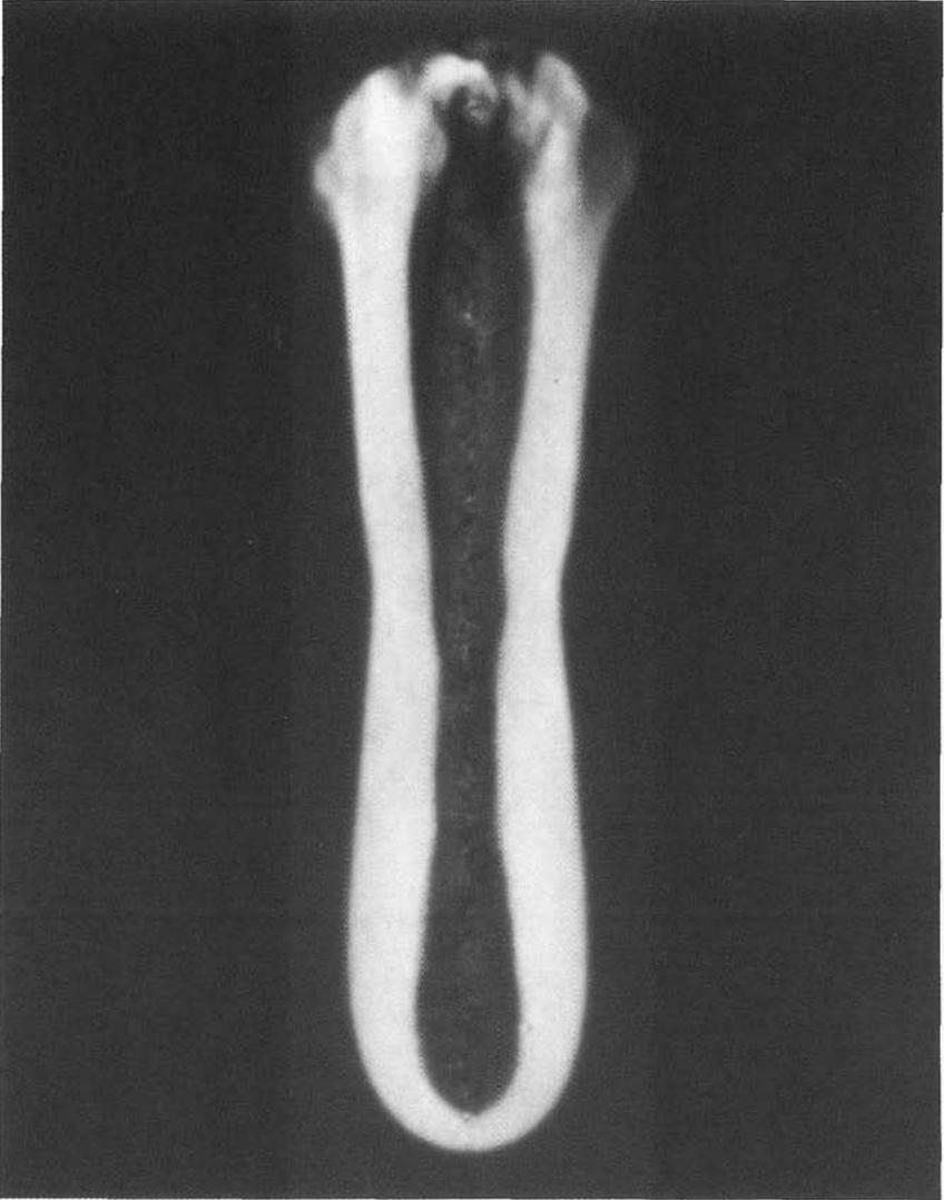
**Fig. 4b** Reconstruction of the cross section of the object derived from Fig. 4a. It shows the void in the middle of the penetrator much more clearly. Hence, the solution is easily realized by peeling the onion from the outside to the inside.
