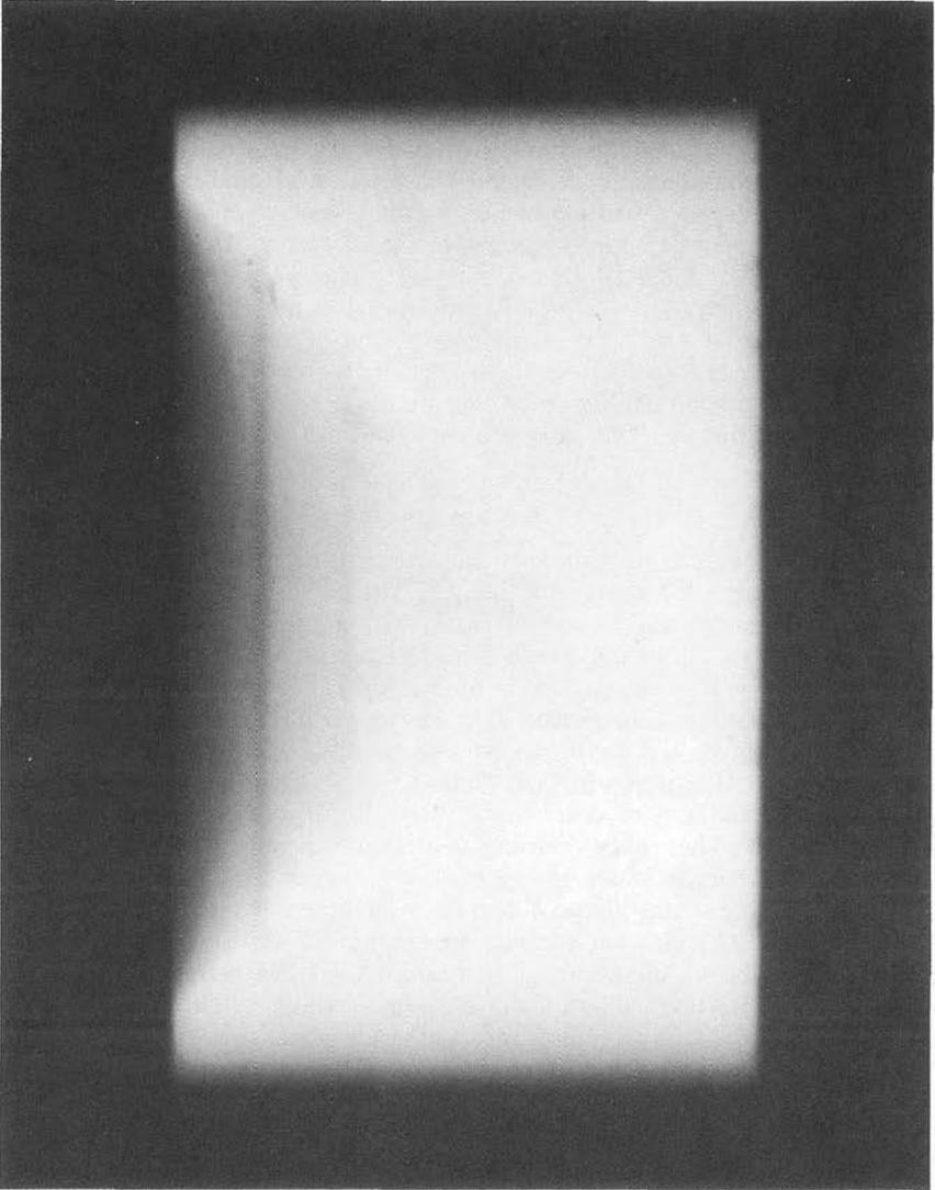
Fig. 3a Radiograph of an axially symmetric steel object taken with a  $\text{Co}^{60}$  source using AA film placed between two 0.25-mm-thick lead screens.
