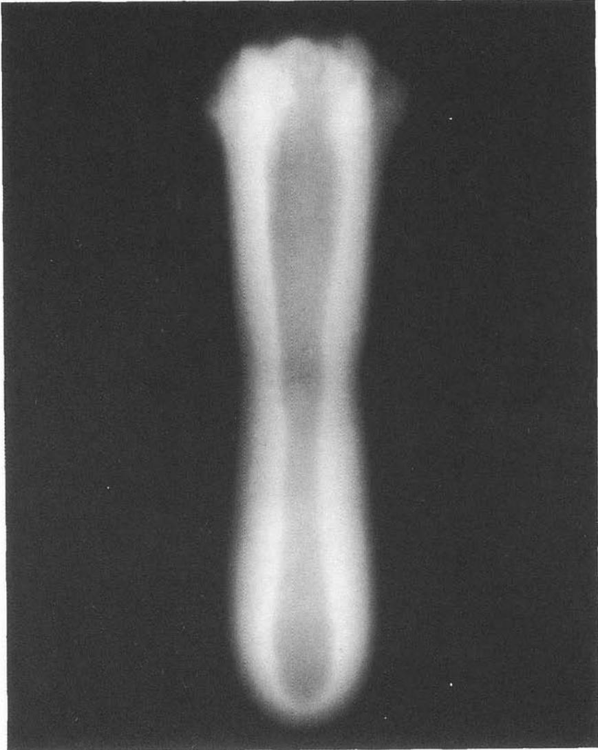
**Fig. 4a** Radiograph of an explosively formed copper penetrator. The penetrator, supplied by Honeywell Corp., was radiographed with a 50-ns-long pulse produced by a 0.8-MeV electron beam. Its velocity was 2.8 mm/ $\mu$ s.
