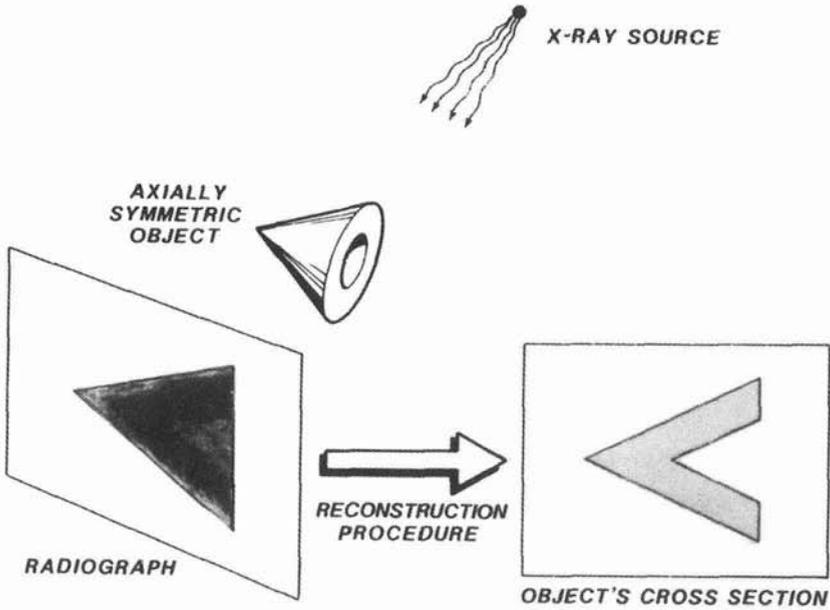
**Fig. 1** Overview of the tomographic method. An object with axial symmetry is radiographed with the radiographic axis perpendicular to the axis of symmetry. The reconstruction procedure transforms the radiograph into an estimate of the cross section of the object.
