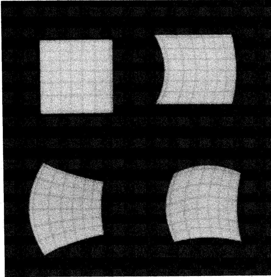
Figure 2: Example of warp achieved through a coordinate transformation consisting of the polynomial warp Eq. (14) including only the quadratic terms. The lower-left image shows a conformal mapping in which the right angles between grid lines are locally preserved.
