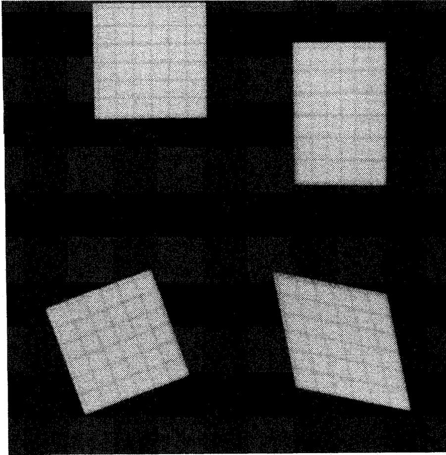
Figure 1: Example of warp achieved through a coordinate transformation consisting of the polynomial warp Eq. (14) including only the constant terms (upper-left) and the linear terms (others). The lower-right image demonstrates the shear effect that occurs when the mapping is not conformal.
