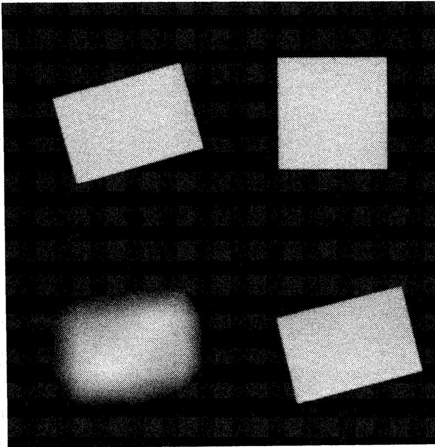
Figure 4: Results for tomographic reconstruction as described in Fig. 3. However, the prior (upper-right) used for the MAP reconstruction (lower-right) is rendered flexible by the proposed warp process that includes the constant and linear terms in Eq. (14). The six warp parameters are determined as part of the reconstruction process.
