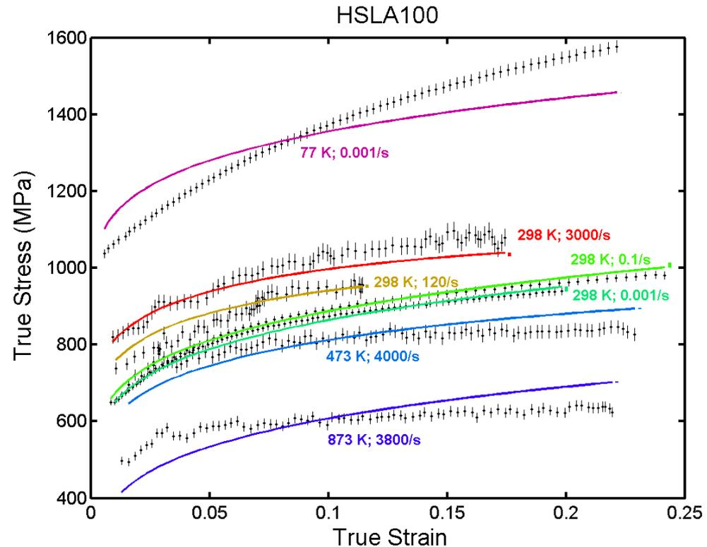
ZA curves include adiabatic heating effect for high strain rates
