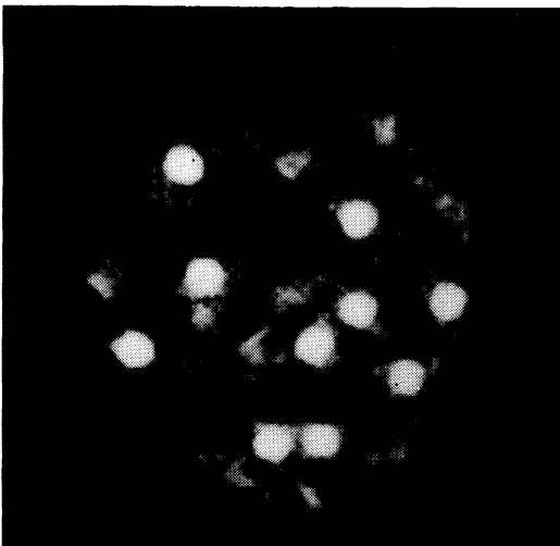
Fig. 3a. Optimized reconstruction of object shown in Fig. 1 from 8 noise-free views after 100 iterations of constrained ART. ( d'=11.69 )
