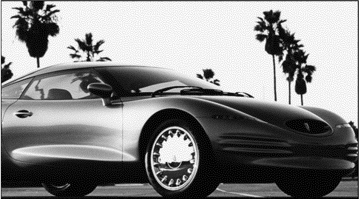
Figure 1. An example of a digital halftone image generated with the direct-binary-search algorithm taken from Ref. 8, which shows the high quality that is achievable with state-of-the-art halftone rendering of gray-scale images. (©IEEE)
